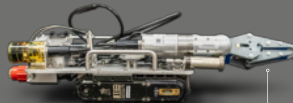
Robotic Clasp used for retrieving loose material
